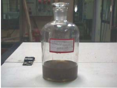
Washing from Intake Manifold and Butterfly Valve
