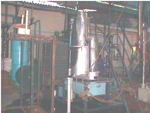
Plate 5: 10 kg/hr gasifier with pine needle briquette
