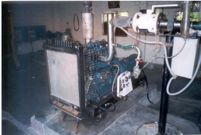
Plate 9.1: The 100% producer gas engine at Dewan Estate
